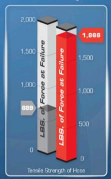
Tensile strength is important if the hose is snagged or stretched.
