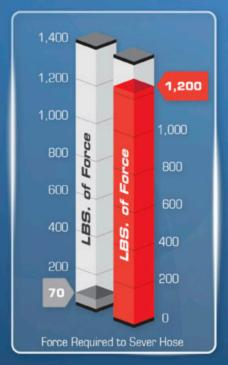
This test simulated a sharp metal object, forced upward between the duals, which can cut or damage the air hose.
